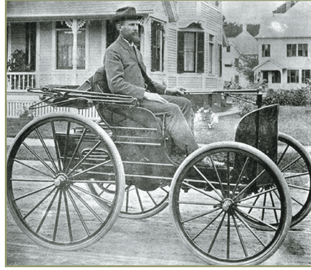
This 2-cylinder water-cooled Duryea motor wagon won the nation's first automobile race on Thanksgiving Day 1895. Racing from Chicago to Evanston, Illinois, and back, the wagon averaged only 7.5 mph.
